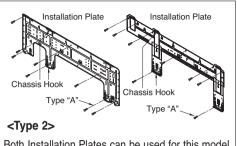
Both Installation Plates can be used for this model.
